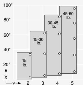
This chart can serve as a guide for determining the number of hinges per door. Note that door weight can also determine the number of hinges required.
