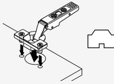
Pre-attached dowels installed with Blum MINIPRESS
