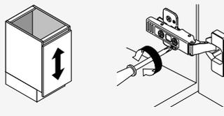
On non-cam mounting plates, loosen screw, adjust door and retighten screws.
