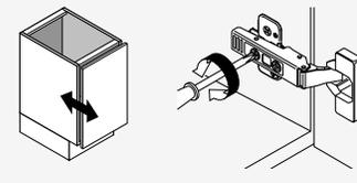
For CLIP, loosen rear screw, adjust and retighten.
