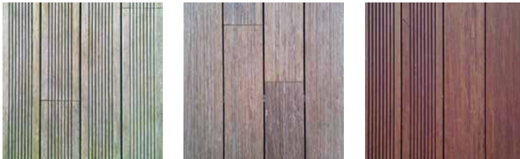
Surface of MOSO® Bamboo X-treme® with different maintenance and cleaning scenarios: weathered, dirty decking (left), weathered, cleaned decking (middle), and refinished decking (right).
