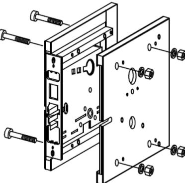
Split clamp plates by removing screws.
