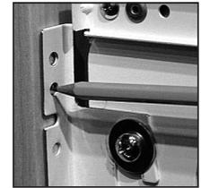
**Step 7:** Carefully pull the door out from the sides and mark several holes on each side through the brackets as a reference in case the tape does not hold the bracket to the door.
