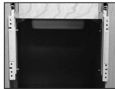
**Step 3:** Peel off one of each of the (2) tape strips provided and carefully place over the door bracket flanges.
