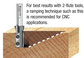
Standard plunge technique or use ramping method as shown to the right.
